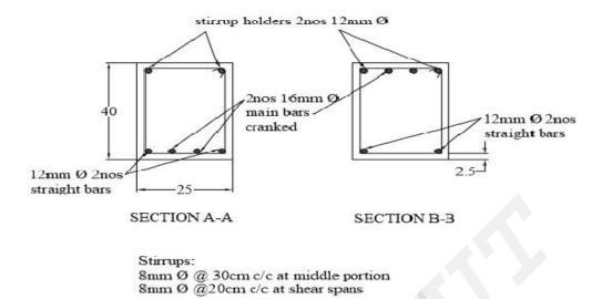
Prepare a bar bending schedule of the simply supported beam of size 25cm x 40cm shown in the figure. (All dimensions are in Centimetres)
