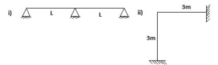
3 a) Find the equivalent joint load matrix for the beam given below. (5)
