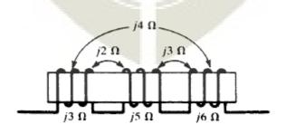
(b) In the circuit shown in figure, find the voltage across the 5  $\Omega$  reactance with the polarity shown.
