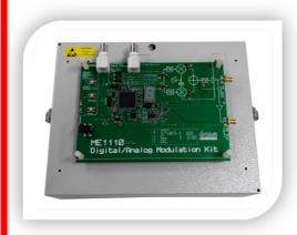
ME1110 Analog/Digital Modulation Board is a versatile system that can produce a variety of digitally modulated band-pass signals. It is also programmed to produce standard analog modulated signals such as AM and FM signals. The default RF (radio-frequency) carrier used by the system is 10 MHz. One of its special features is
