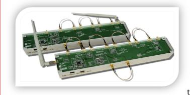
ME1000 Transmitter – Receiver Kit: Transmitter is an electronic device which generates a radio frequency alternating current. When a connected antenna is excited by this alternating current, the
